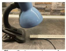
Place the temperature probe under the metal ruler
