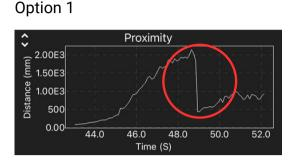
If the track's incline angle is steep, you may observe significant changes in distance on the graph.
