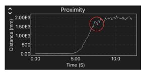
If the platform's incline angle is small, you won't notice significant changes on the distance graph.
