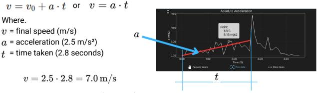
The car's speed at the end of the platform is 7.0 m/s.
