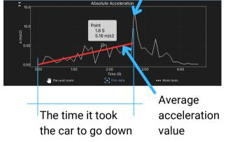
For more accurate data, run the toy car several times, fill in the table and calculate the average acceleration. Do not change the platform inclination angle.
