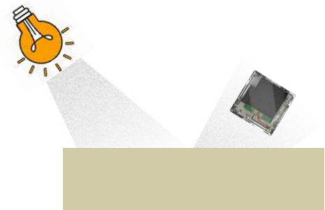
Measuring RGB scale of cardboard from the reflected light
