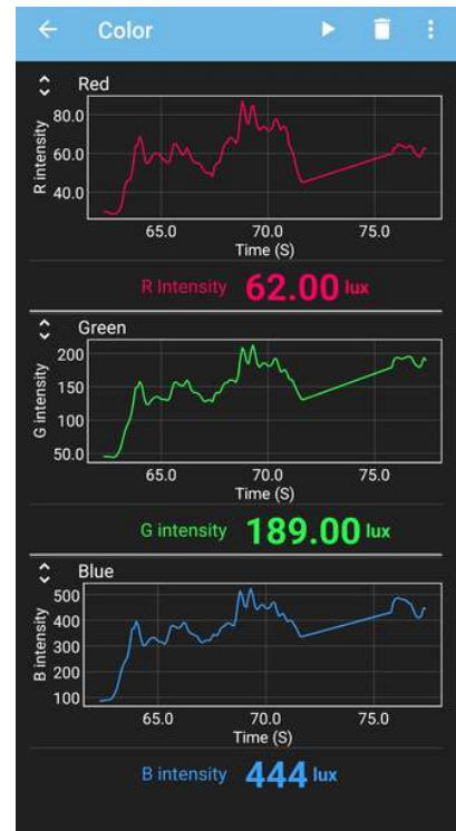
Measuring RGB scale of cardboard from the reflected light
