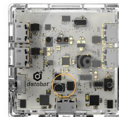
The Air Pressure sensor is a black square chip labeled hPa for hectopascals.
